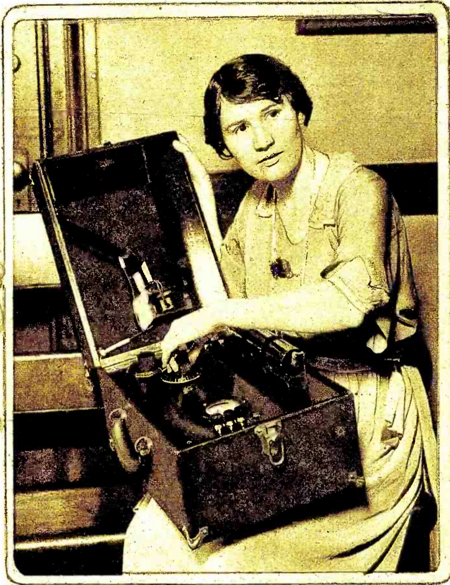
This Unique and Compact Receiver Made an Excellent Showing at the New York Radio Show. Reception was Accomplished with a Loop.
