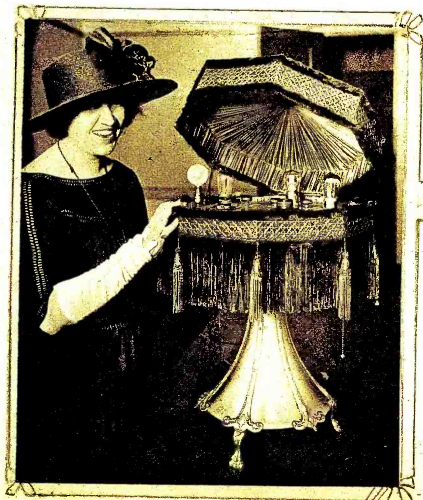
Excellent Results Have Been Obtained with This Handsome, Self-Contained Radiophone Receiver Exhibited at the Last New York Show. The Aerial, Batteries, Amplifier and Loud-Speaker are All Inside the Cabinet.
