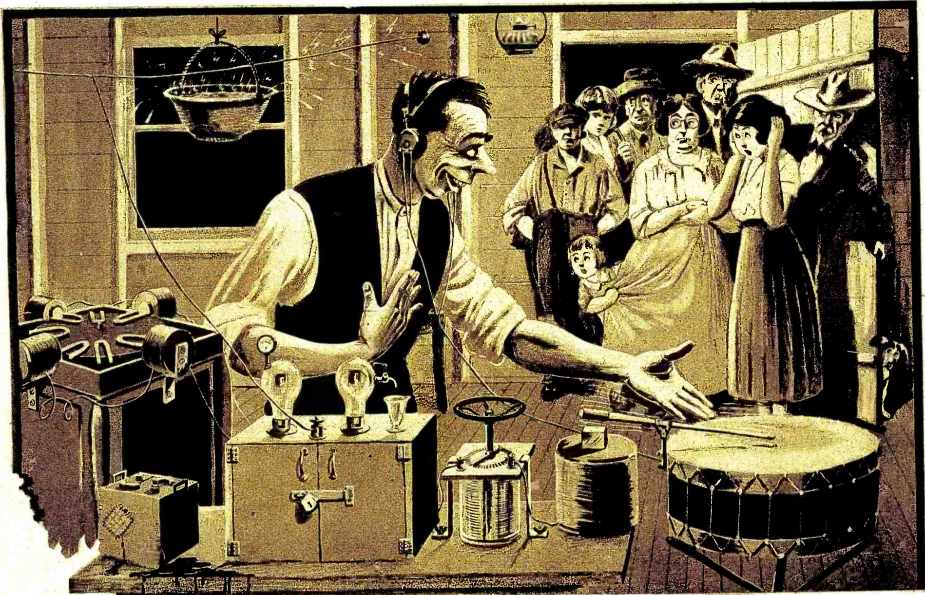
I Constructed an Electromagnet and Put It in Series With the Receiver, Which Would Not Sound, Due to the Weakness of the Currents. I Purchased a Large Drum and Drumsticks of Laminated Iron, and Hinged Them So That the Pull of the Electromagnet Would Cause the Drumsticks to Strike the Drum, and Thus Reproduce the Signals.
